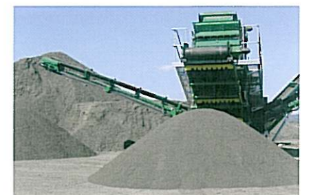
Discharge conveyors with a very high discharge height for maximum stockpiling capacity
