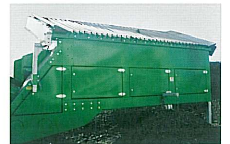
Wide feed hopper with tipping grid
