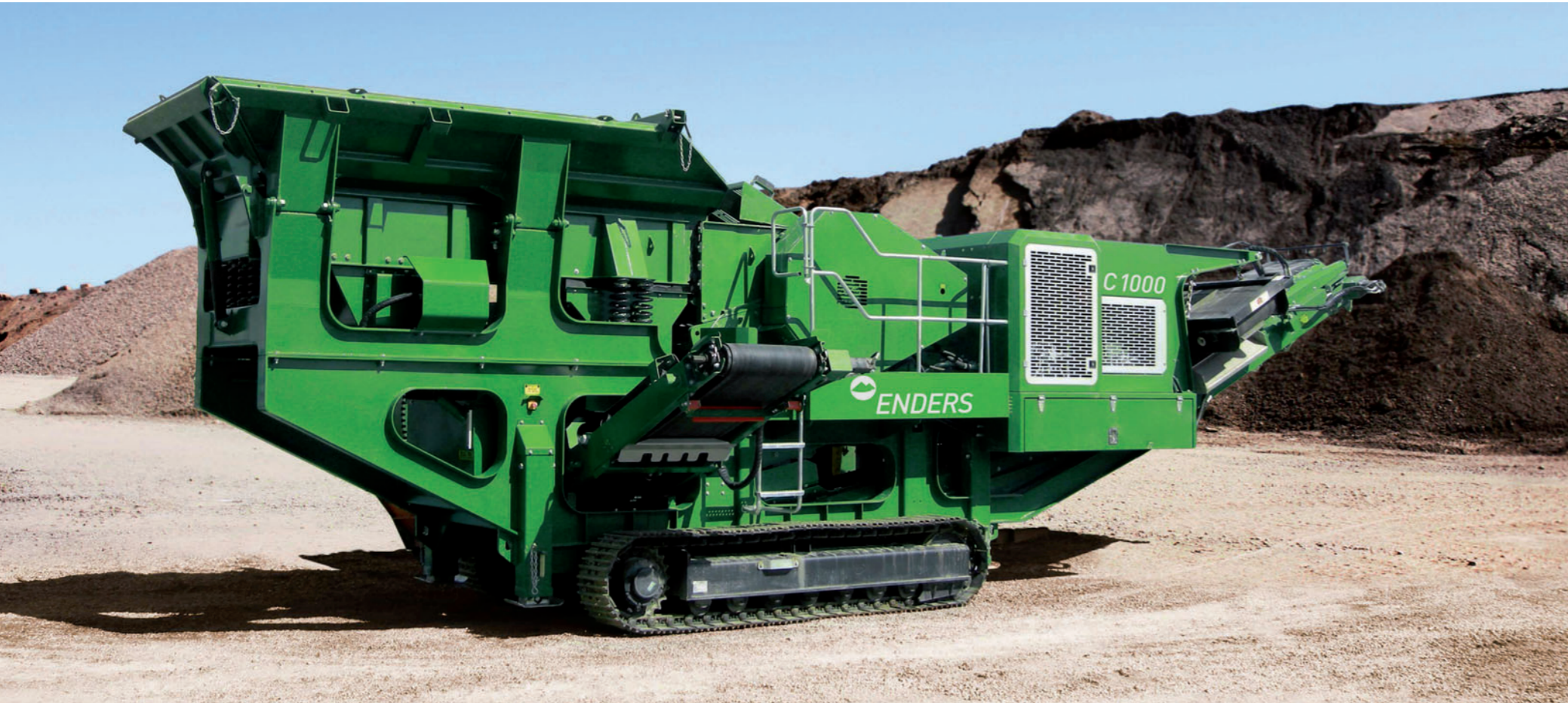
Hydraulic feed hopper with a capacity of 5.4 m 3 and a variable-speed vibration feeder
