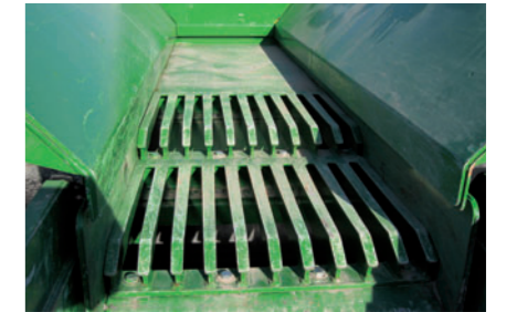
Hydraulic feed hopper with a capacity of 5.4 m 3 and a variable-speed vibration feeder
