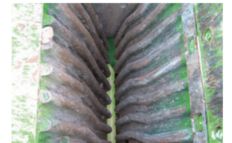
Crusher inlet approx. 1,016 x 610 mm
