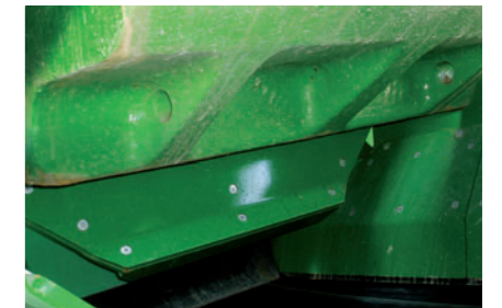
Adjustable plate for deflecting rebars
